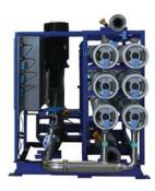
In December 2008, Pure Aqua successfully supplied a skid-mounted Industrial Brackish Water Reverse Osmosis (BWRO) system to produce 50m<sup>3</sup>/hr product at 77°F using (42) 8"x40" FILMTEC LE-440i membrane elements, (6) FRP pressure vessels 7 elements per each vessel, SS multistage pump, PLC based controls and a digital conductivity and ORP read out, 380V/3ph/50Hz.
