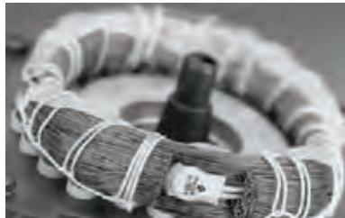
**Fig. 46** Thermal switch incorporated in windings
