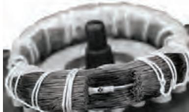
**Fig. 44** PTC sensor incorporated in windings
