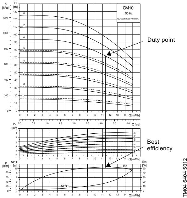
**Fig. 32** Example of a CM pump's duty point
