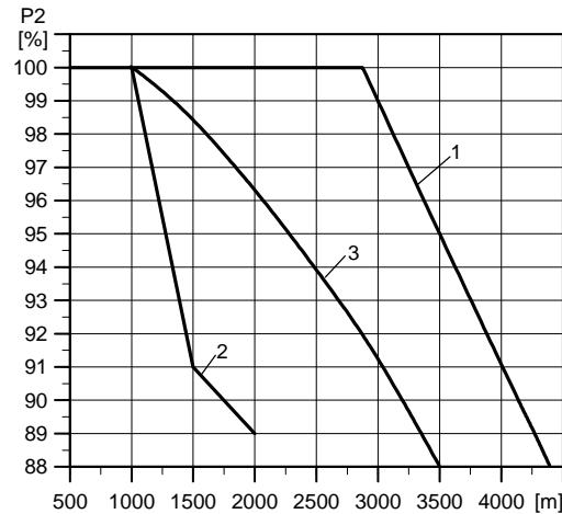
Fig. 10 Relationship between motor output ( $P_2$ ) and altitude
