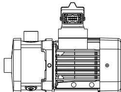
Fig. 36 Motor with multiplug connection
